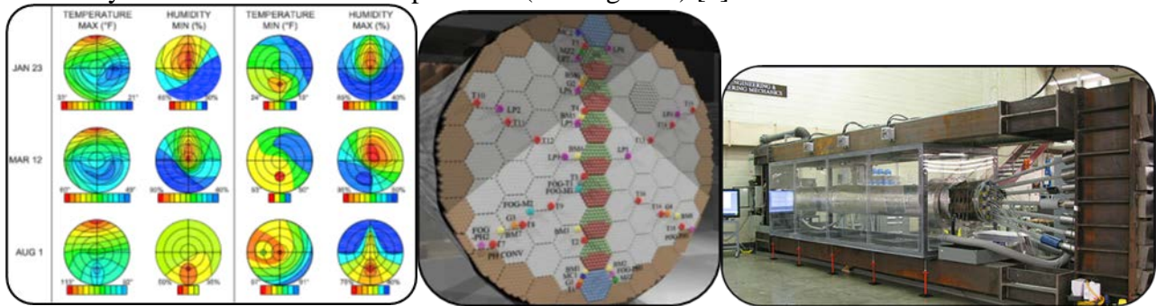
Figure 6: Cable corrosion research and dehumidification utilizing internal sensors on full scale cable mock-up at Columbia University
