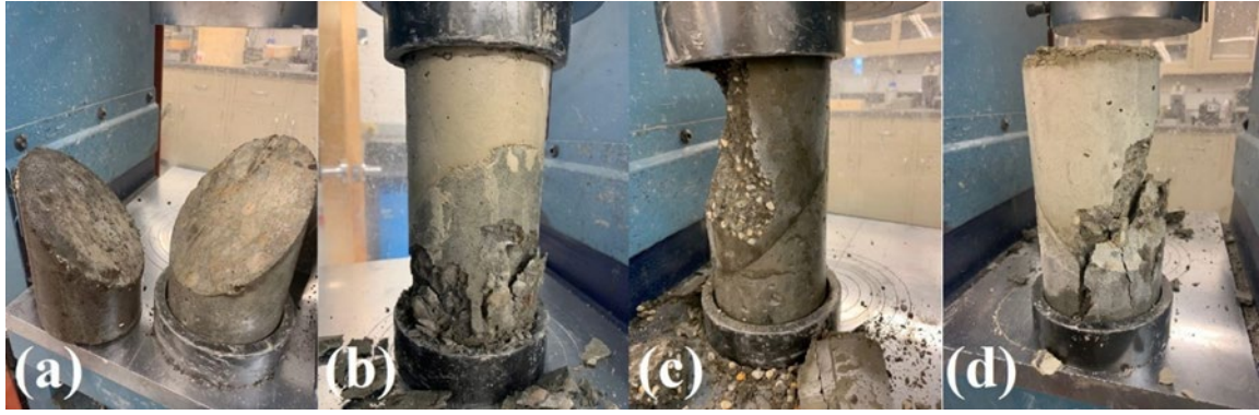
Figure 4: Failure modes observed in the slant shear bond strength tests: (a) Bond failure, (b) Substrate concrete failure, (c) Repair material failure, and (d) Combination of failures
