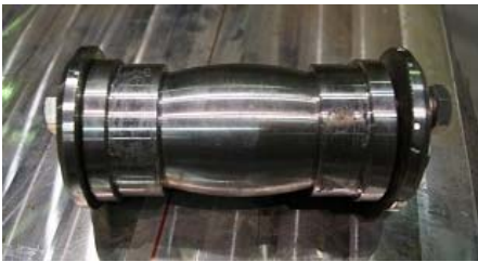
Fig. 6.1. Spherical pin after test
